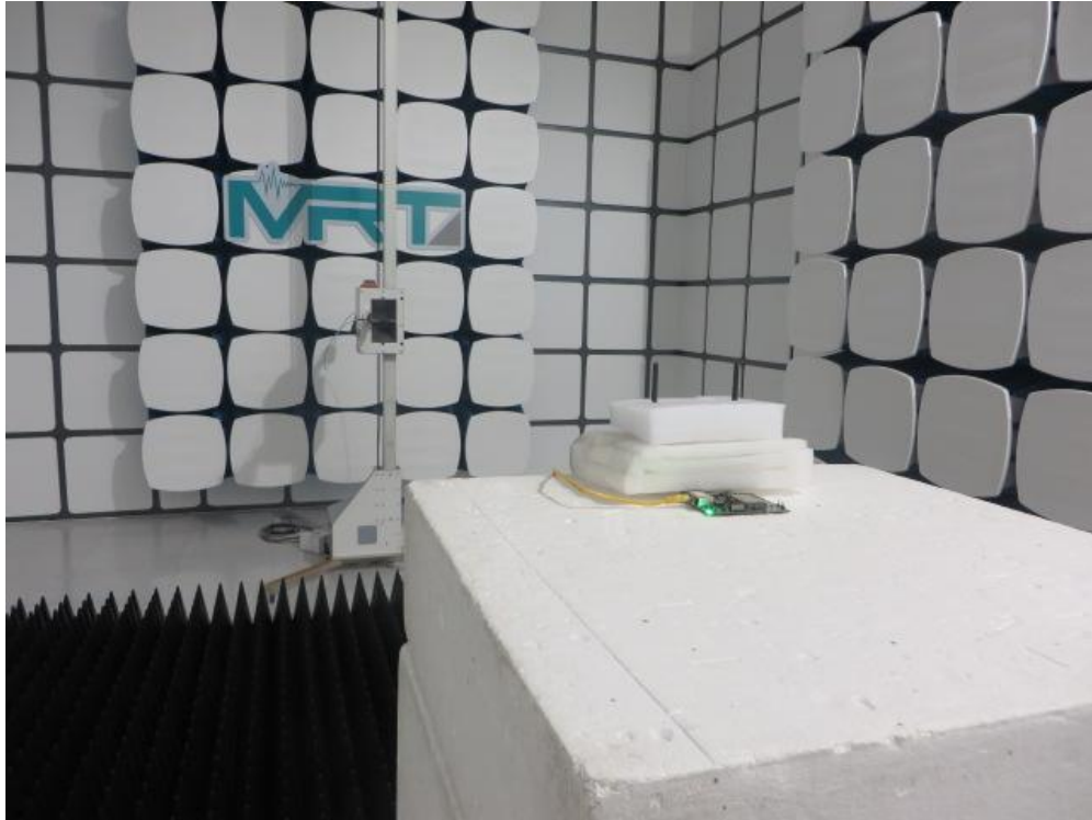
Description: Radiated Emission Test Setup for 18GHz ~ 40GHz for Dipole Antenna 1#
