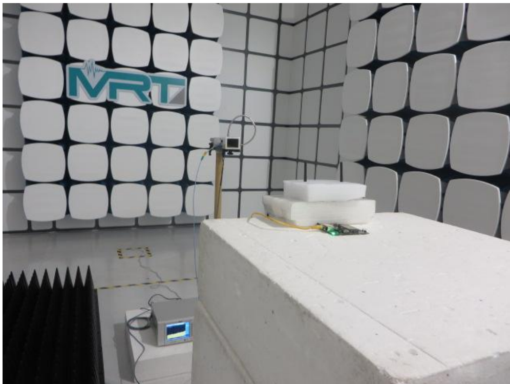
Description: Radiated Emission Test Setup for 18GHz ~ 40GHz for Dipole Antenna 1#
