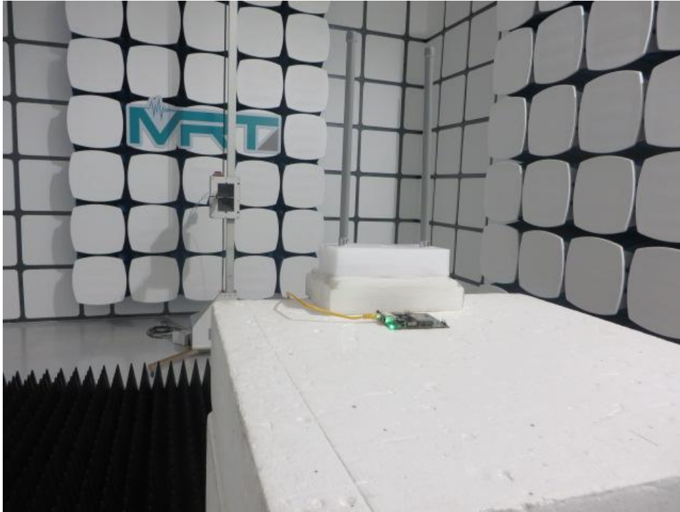
Description: Radiated Emission Test Setup for 18GHz ~ 40GHz for Panel Antenna 2#
