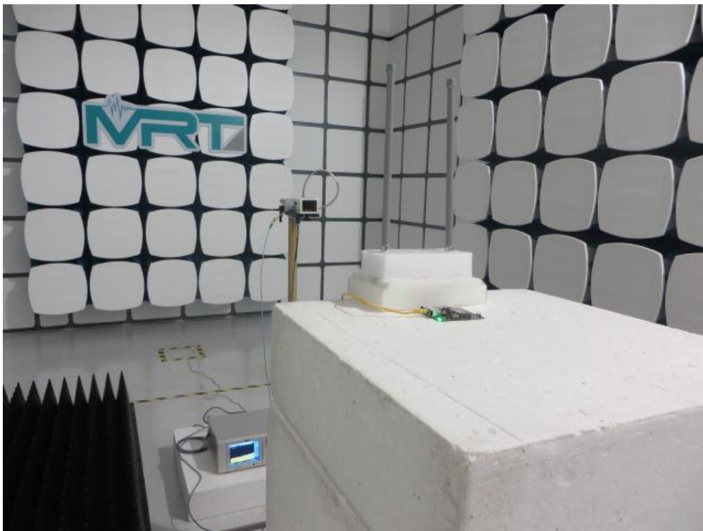
Description: Radiated Emission Test Setup for 18GHz ~ 40GHz for Panel Antenna 2#
