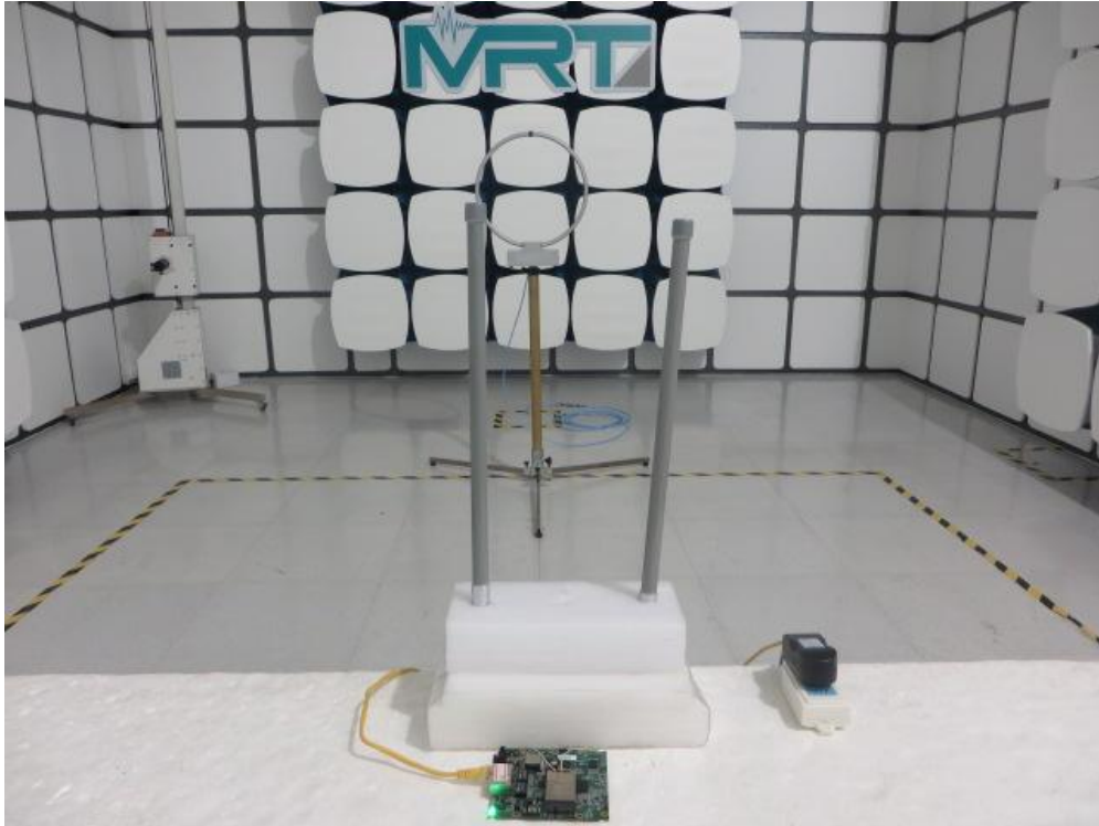
Description: Radiated Emission Test Setup for 30MHz ~ 1GHz for Panel Antenna 2#
